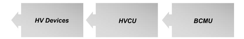
HV devices include relay, contactor, fuse, DC switch, pre-charging resistor and current sensor;
